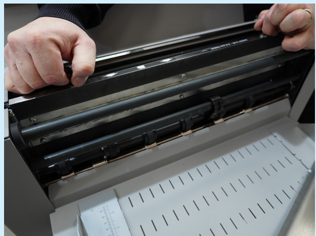
Images showing the removal of 'EasyBlade quick release mechanism'.
